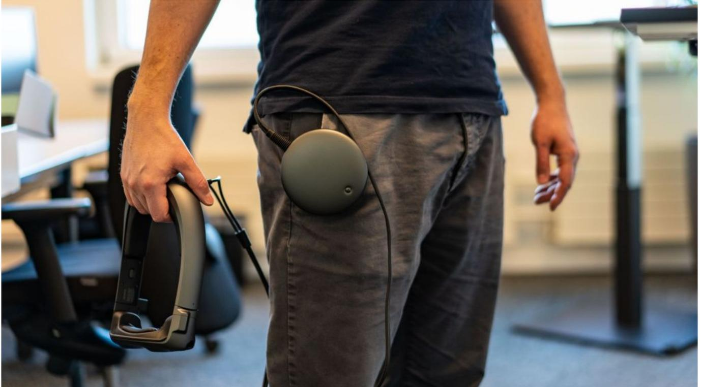
While the “Lightwear” glasses only contain the visualization and sensors, the actual hardware for computation and the battery are stowed away in the “Lightpack”. (Zühlke/Simon Ziffermayer)
